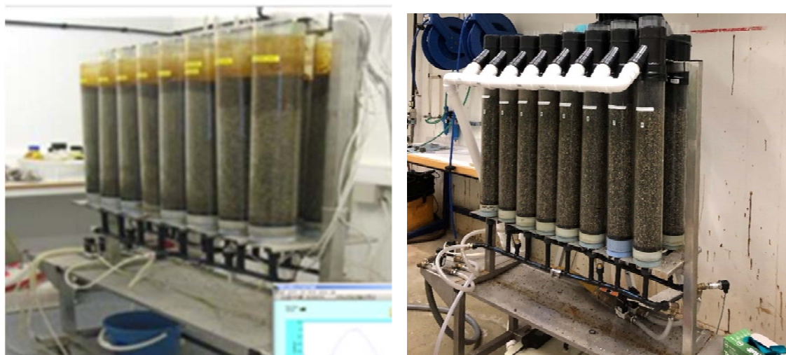
Figure 1.1 Sediment column systems: Previous system (left photo) and modified system used in current project (right photo).
