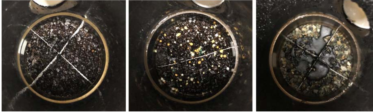
Figure 2.3 Surface of columns at day 0: From left to right: COL9 (18 g oil and 1 g fertilizer premixed with sediment), COL12 (18 g oil premixed with sediment and 3 g fertilizer applied on surface), and COL16 (6 g oil on surface, no fertilizer).
