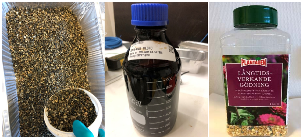
Figure 2.1 Sediment, oil and fertilized used in the column systems.
