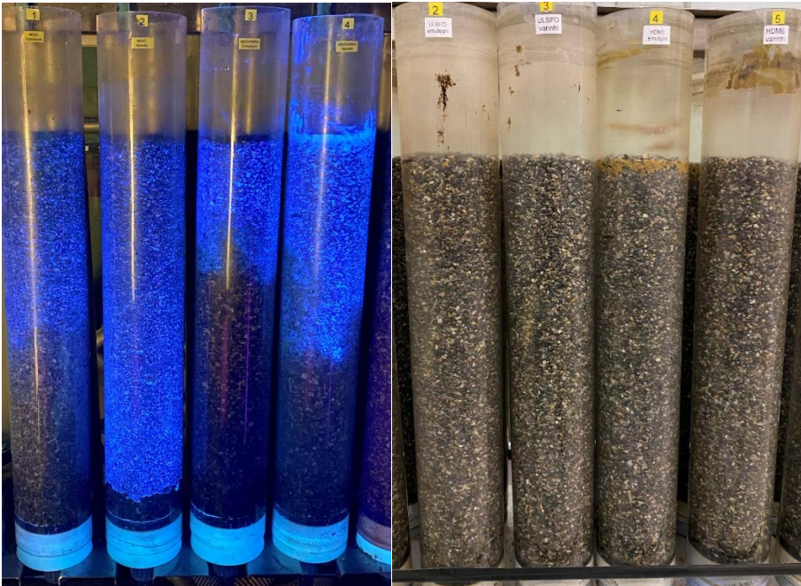
Figure 4-1 Pictures of the sediment columns holding the different fuel oils after 8 tidal cycles. The oils are in the following order from left to right: MGO 250 °C+ emulsified, MGO 250 °C+, WRG emulsified, WRG, ULSFO emulsified, ULSFO, HDME 50 emulsified and HDME 50.
