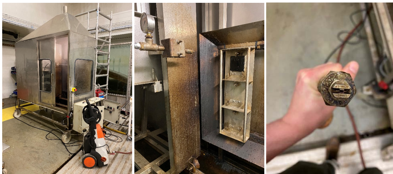
Figure 3-15 Pictures showing the Flushing Robot, the steel rack holding the tiles and the nozzle.
