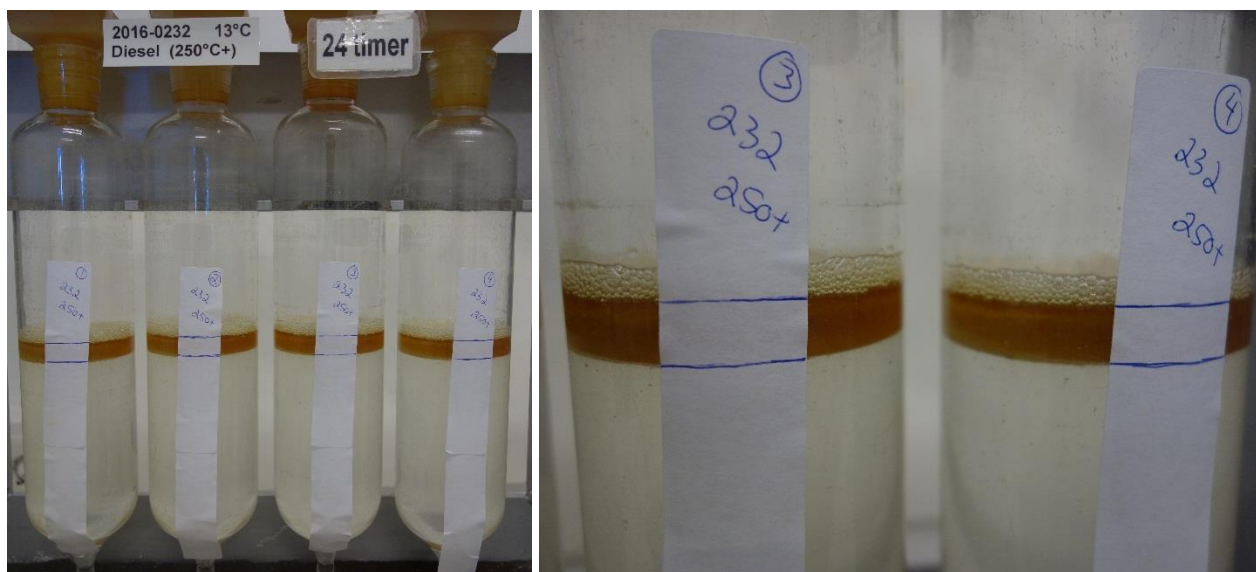
Figure 5-8: Rotating cylinders containing weathered 250°C+ residue of Rotterdam diesel after 24 hours of rotation. The black lines on the white marks indicate the volume of water-free oil used in the test, and coloured lines show changes during the 24 hours of rotation. No significant water uptake was observed.
