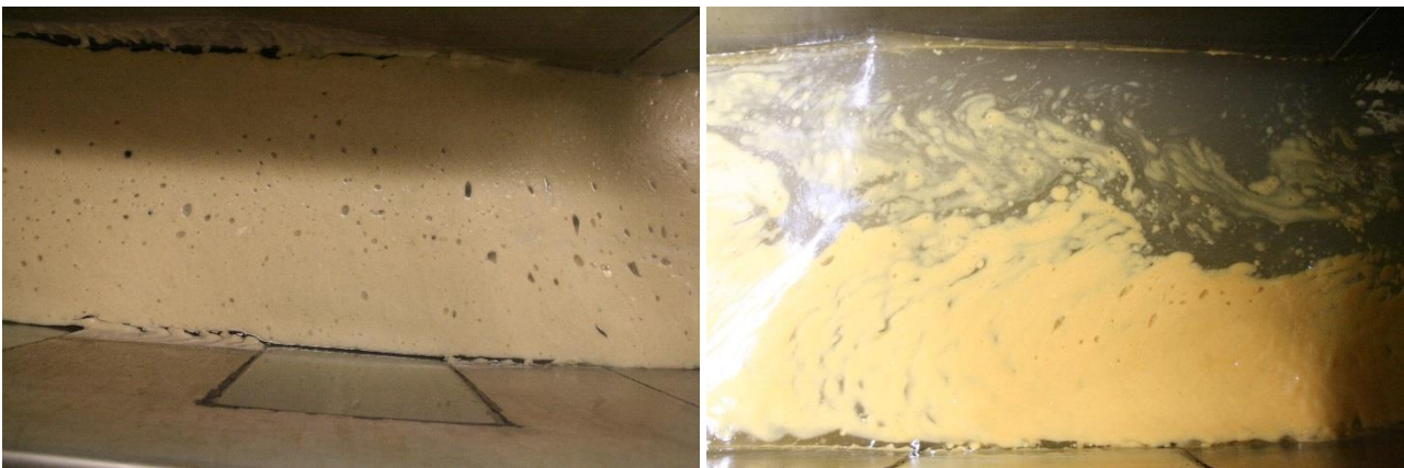
Figure 5-11: Show the emulsion of WRG after 72 hours of weathering in the flume, prior to dispersion. Emulsion from testing at 2 °C is shown to the left, and emulsion from testing at 13 °C is shown to the right
