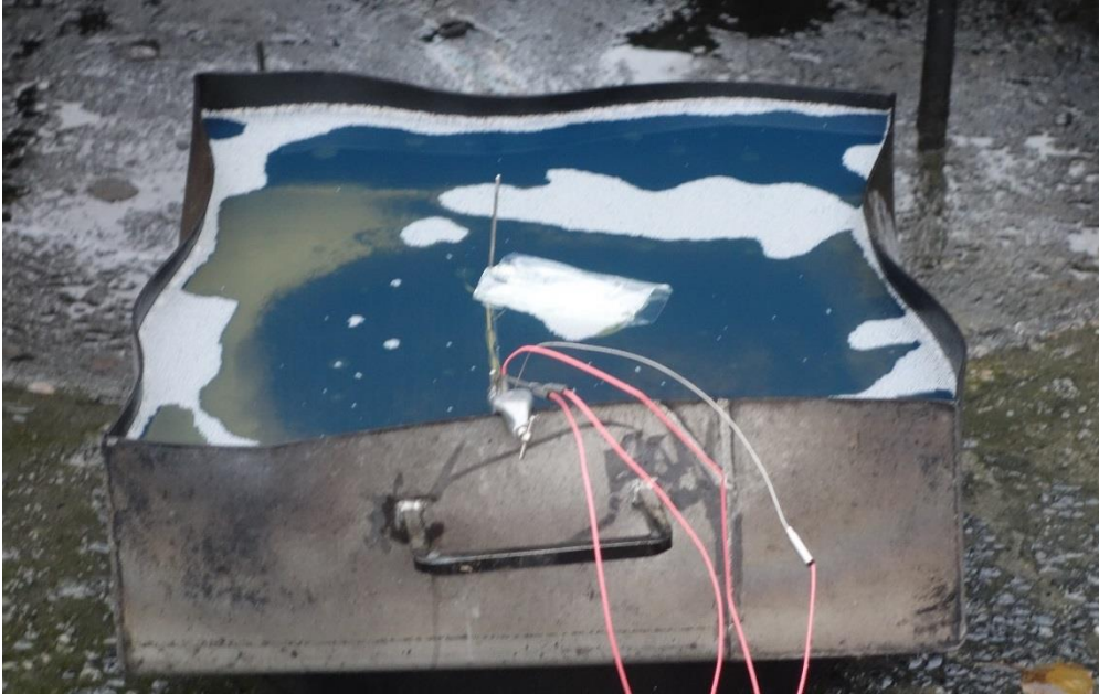
Figure A-8: Basin used for up-scaled testing, shown with sensors for flame temperature, oil temperature and water temperature.
