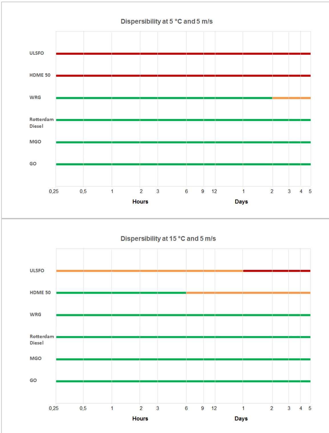
Figure 7-2: Predicted dispersibility over time at 5 and 15 °C for 5 m/s wind, for all tested oil. Green = dispersible, orange = reduced dispersibility and red = not dispersible.
