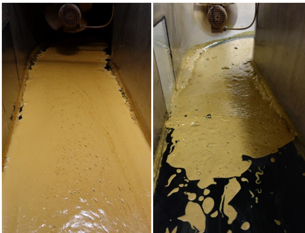
Figure 5-15: Emulsions of HDME 50 after 72 hours of weathering, prior to dispersion. The homogenous emulsion (20232 mPa·s) that formed at 13 °C is shown to the left, while the right hand picture show the emulsion (18730 mPa·s) at 2 °C, which contained solidified oil.
