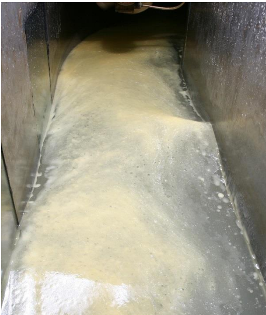
Figure 5-7: The emulsion like layer formed by MGO at 13 °C in the meso-scale flume experiment
