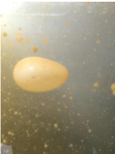
Figure 5-10: Example of structure observed in the water column, assumed to be a water droplet covered by an oil/emulsion "skin". The large bulb was estimated to have a diameter of 2-3 cm.
