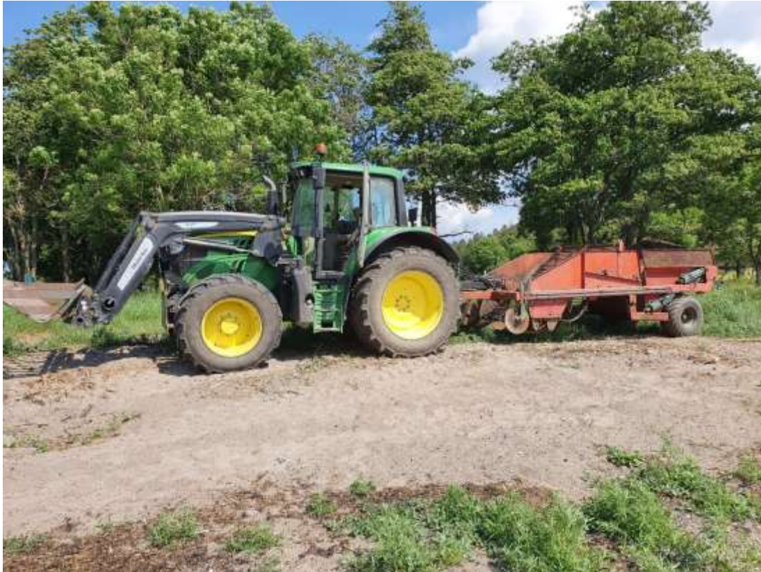
Figure 23. Tractor sieving with equipment that had too great a gap between the gratings.
