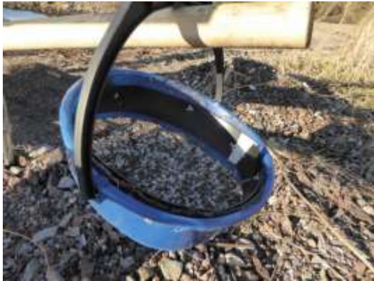
Figure 24. A modified bucket with a mesh can be used as a sieve.
