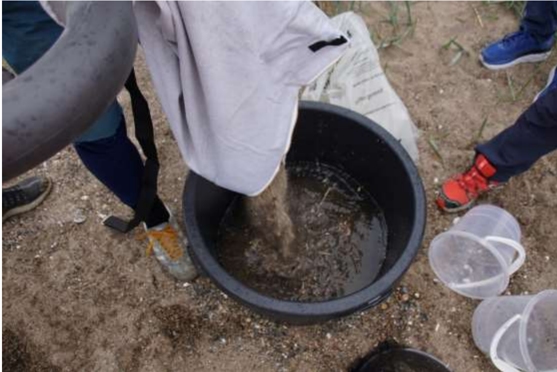
Figure 15. Emptying a vacuum cleaner bag straight into a water bath.
