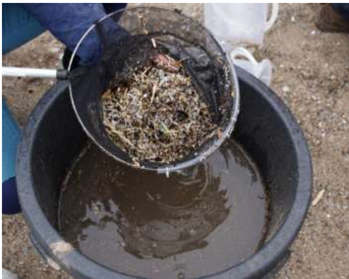
Figure 10. After sieving, a bucket water bath is used when the particle size is similar to the pellets.
