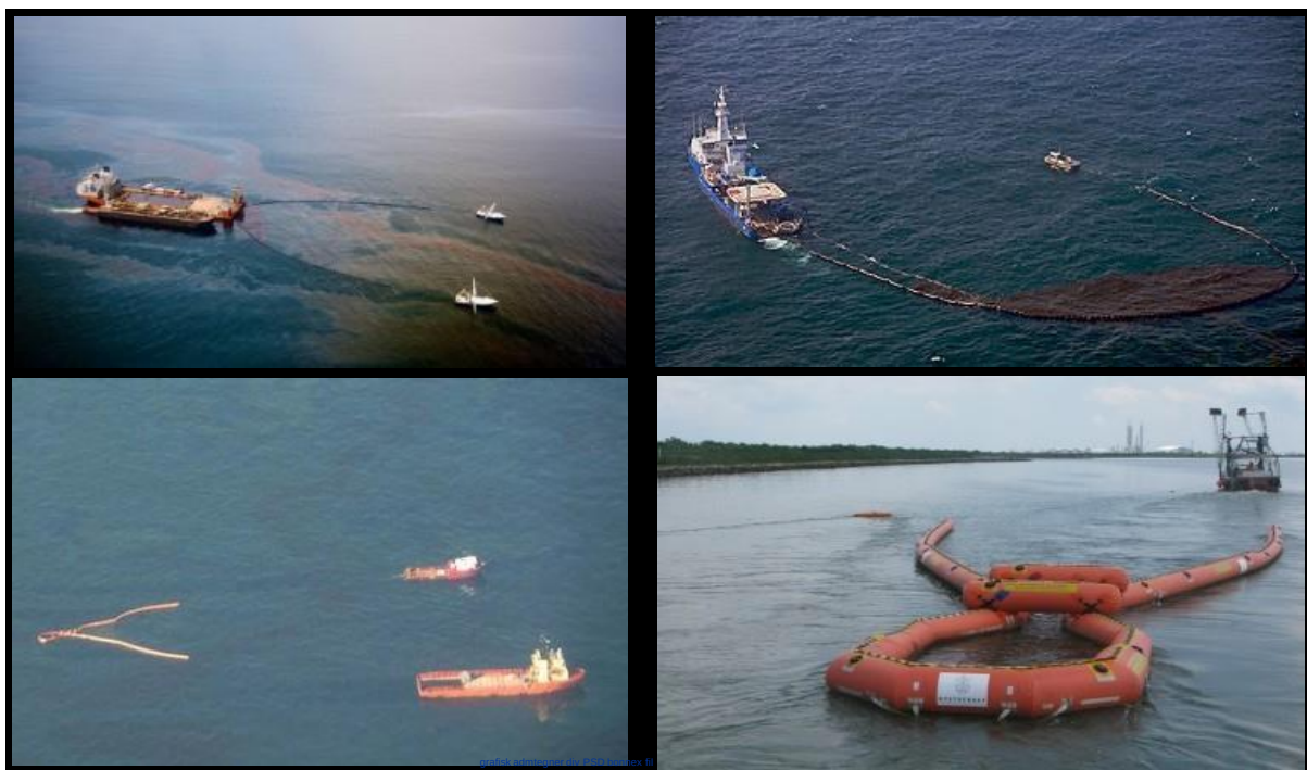
Figure 4-4 Examples of mechanical recovery systems involved in the response (offshore).
