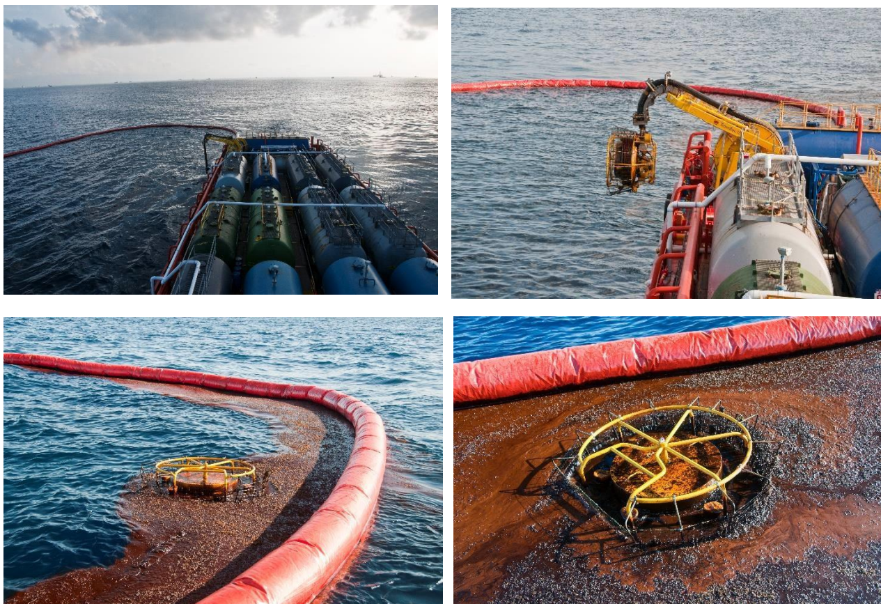
Figure 4-11 Upper: The No-800 was operated in a "J- configuration" from Ella G. Down: "Chicken wires" mounted around the skimmer to enhance the flowability of the emulsion into the weir.
