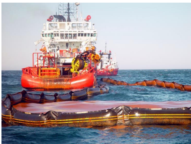
Figure 4-19 Emulsion confined in a boom ready for recovery by the Transrec system onboard "Skandi Stord."
