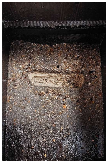
Fig. 1: Full penetration of a fluid LSFO in sandy sediment.
