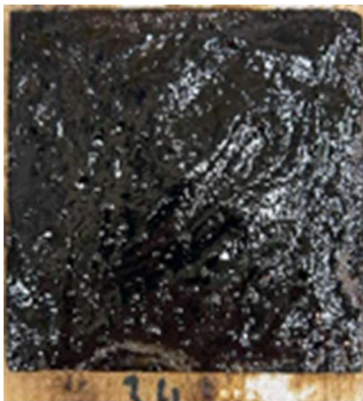
Fig.4: Slate tile covered with a LSFO and washed at 25°C/50 bar after addition of a surface cleaning agent
