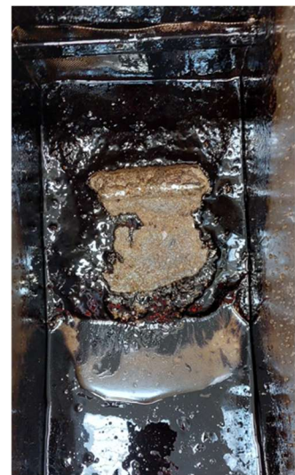
Fig. 2: Semi-solid LSFO on sandy sediment. Can be rolled and leave the sediment clean.
