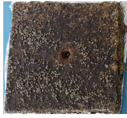
Fig.5: Granite tile covered with a LSFO (left) and let for natural degradation for 11 months (right). Oil elimination and colonisation by barnacles is observed.
