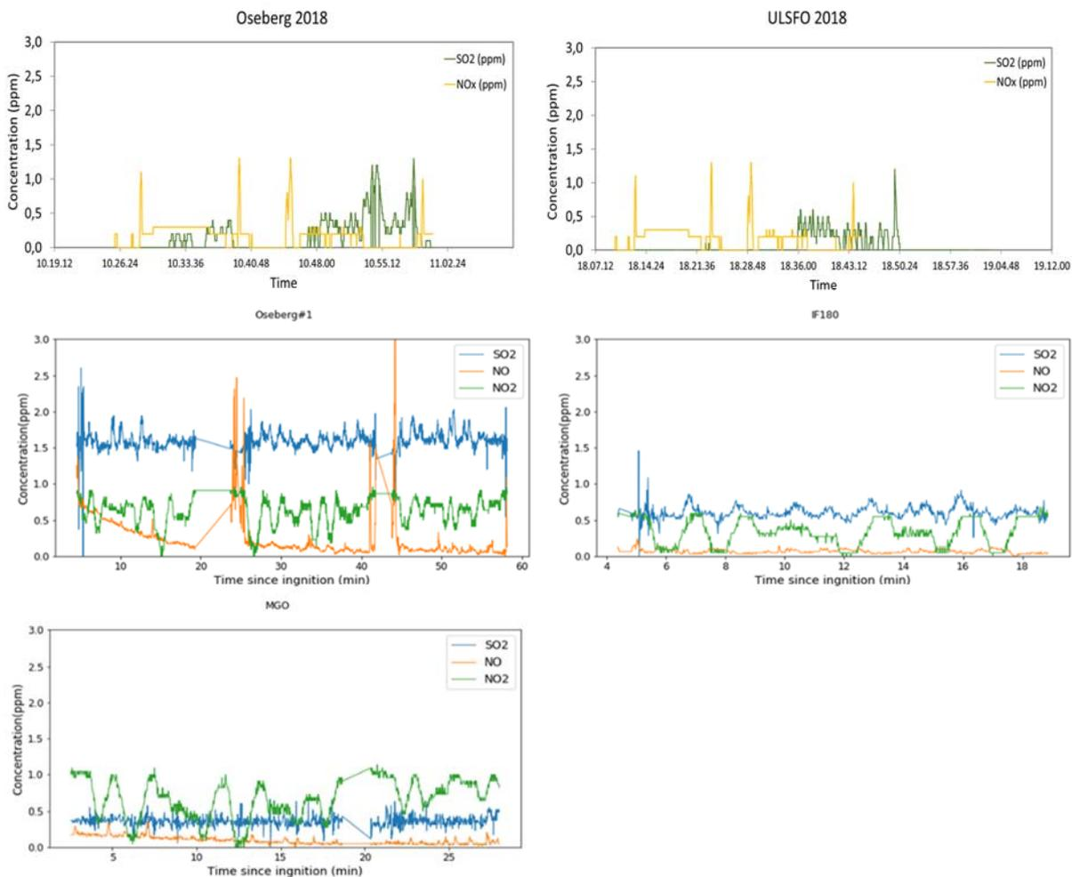
Figure 3.8 Measured concentrations of SO<sub>2</sub> (green lines), NO<sub>x</sub> (2018) and NO (yellow lines), and NO<sub>2</sub> (2019, blue lines) in the smoke plume. Gas monitoring data from Oseberg Fireboom (Oseberg#1) in 2019, not from Oseberg Pyroboom (Oseberg#2). Different sensors were used in 2018 and 2019.
