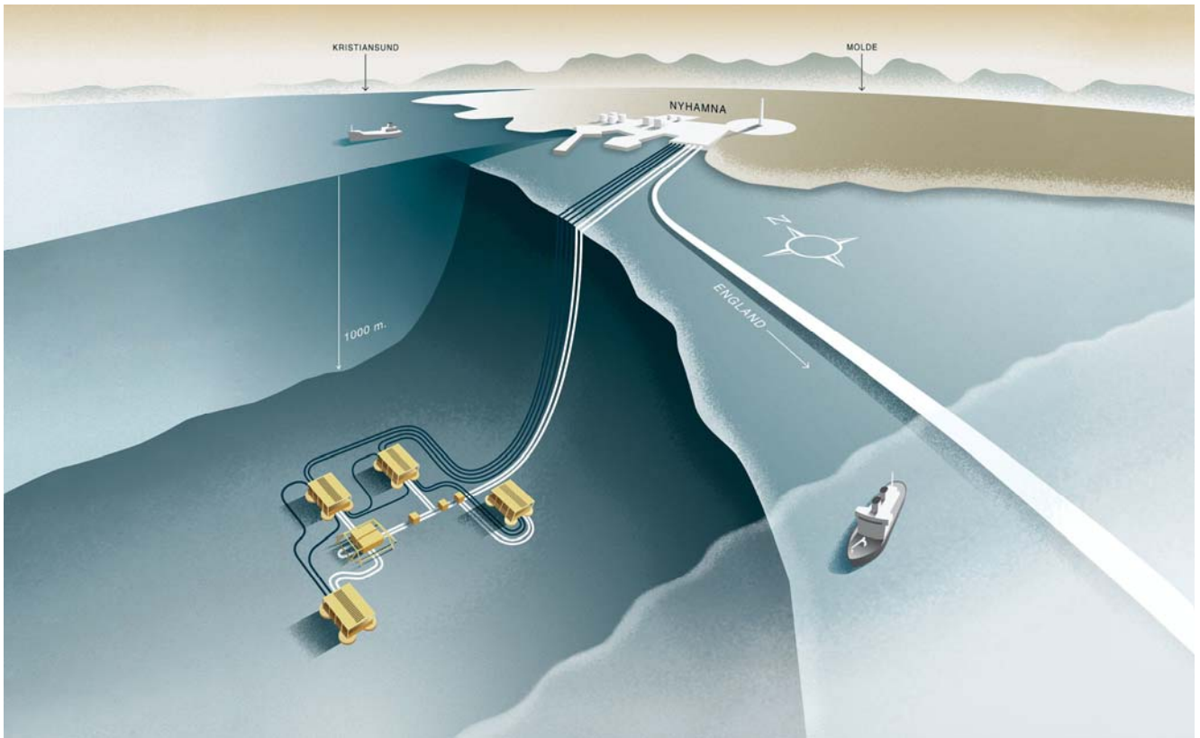
Figure 1: © Norsk Hydro - Illustration of the Ormen Lange natural gas complex, showing the subsea production installations, the process plant and the export pipeline to the UK.
