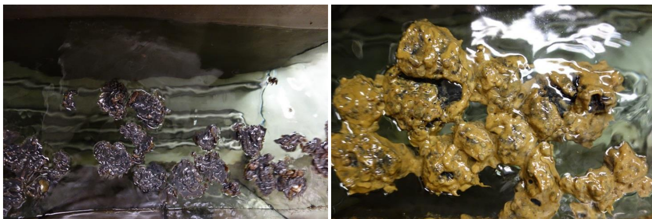
Figure 2-9: immediate solidification (right, 0 hr) and emulsification on surface of waxy lumps (right, 4 hr)
