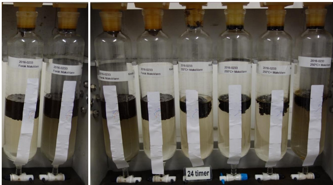
Figure 2-9: Rotating cylinders expressing the emulsifying properties of fresh and weathered ULSFO (four parallels of each) after 24 hours of rotation at 2 °C.
