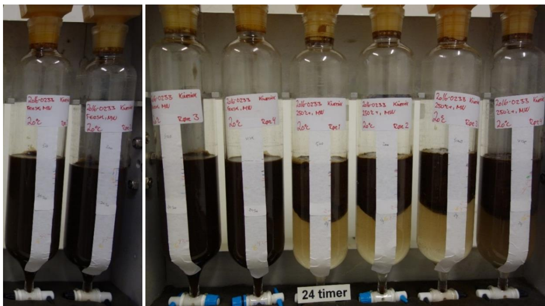
Figure 2-11: Rotating cylinders expressing the emulsifying properties of fresh and weathered ULSFO (four parallels of each) after 24 hours of rotation at 20 °C
