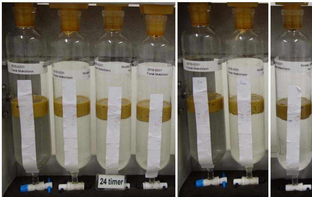
Figure 2-6: Rotating cylinders expressing the emulsifying properties of HDME 50 after 24 hrs rotation (left) and application of emulsion breaker (middle and right), at 2 °C. The dosages of emulsion breaker were 500 ppm and 2000 ppm, with a reference emulsion to the far right.
