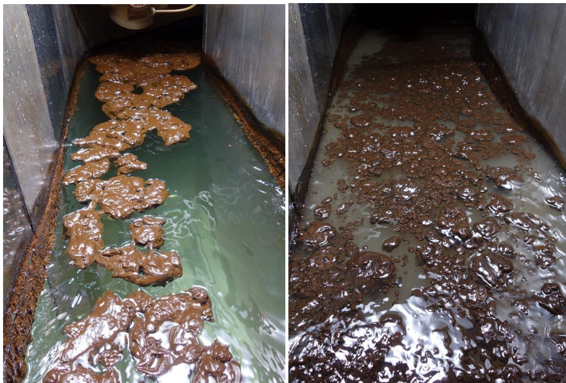
Figure 3-3: Emulsion prior to dispersion (left, 72 hr) and after the second dispersion (right, 72 hr + 2 disp.)
