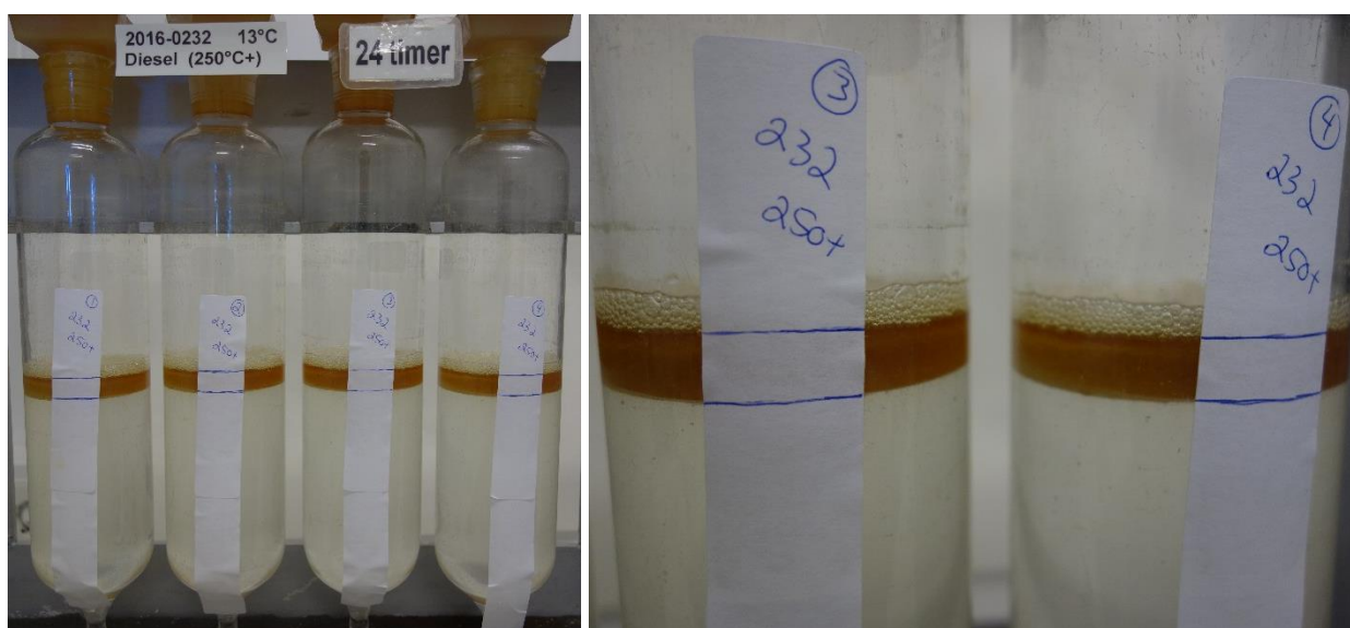
Figure 2-5: The rotating cylinders containing Rotterdam Diesel after 24 hr rotation. The close up to the right show the foam that formed during rotation, and also show the lack of total volume increase due to lack of emulsification.
