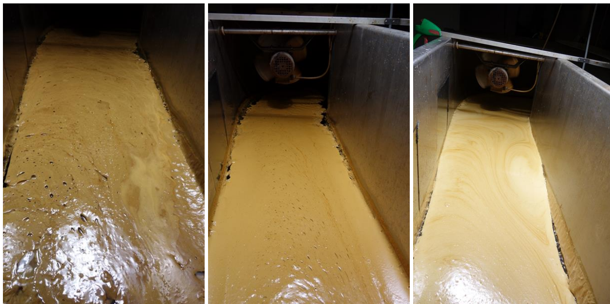
Figure 2-3: Lighter coloured emulsion (left, 6 hr), emulsion prior to dispersion (middle, 72 hr) and after the second application of dispersion (right, 72 hr + 2 disp)
