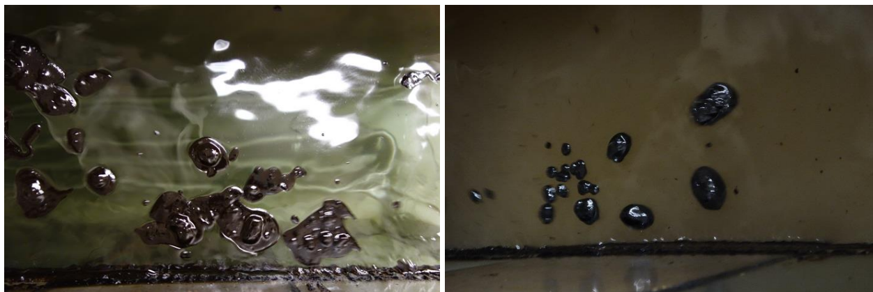
Figure 3-10: Emulsion and waxy lumps prior to dispersion (left, 72 hr) and waxy lumps after the second dispersion (right, 72 hr + 2 disp.)
