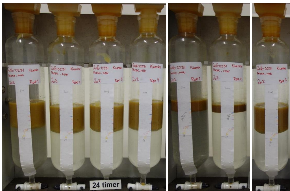
Figure 2-8: Rotating cylinders expressing the emulsifying properties of HDME 50 after 24 hrs rotation (left) and application of emulsion breaker (middle and right), at 20 °C. The dosages of emulsion breaker were 500 ppm and 2000 ppm, with a reference emulsion to the far right.
