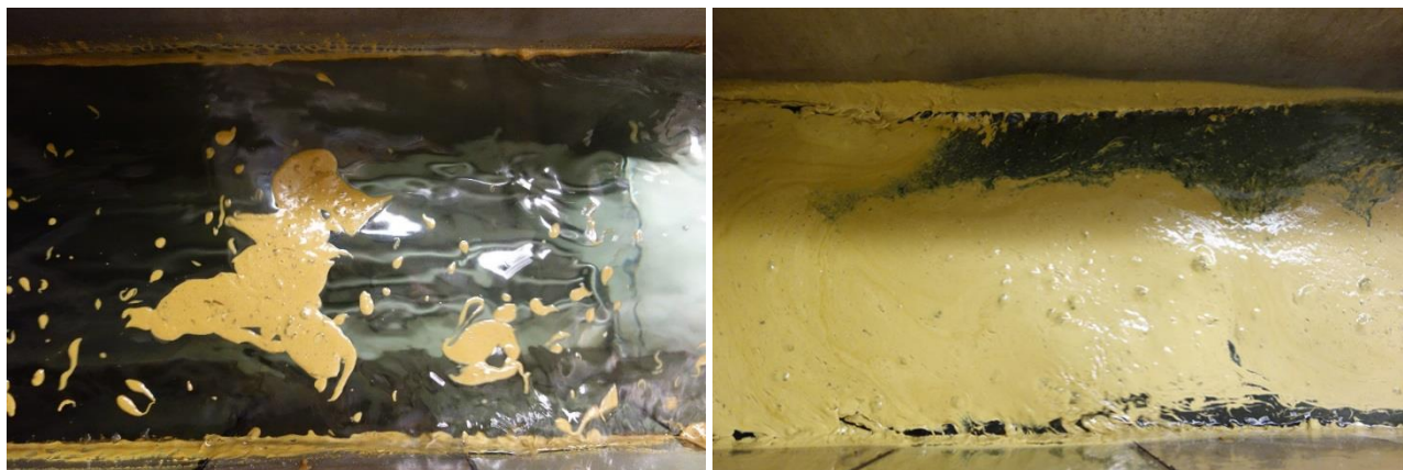
Figure 2-10: emulsion with wax lumps prior to dispersion (left, 72 hr) and emulsion after second dispersion (right, 72 hr + 2 disp)
