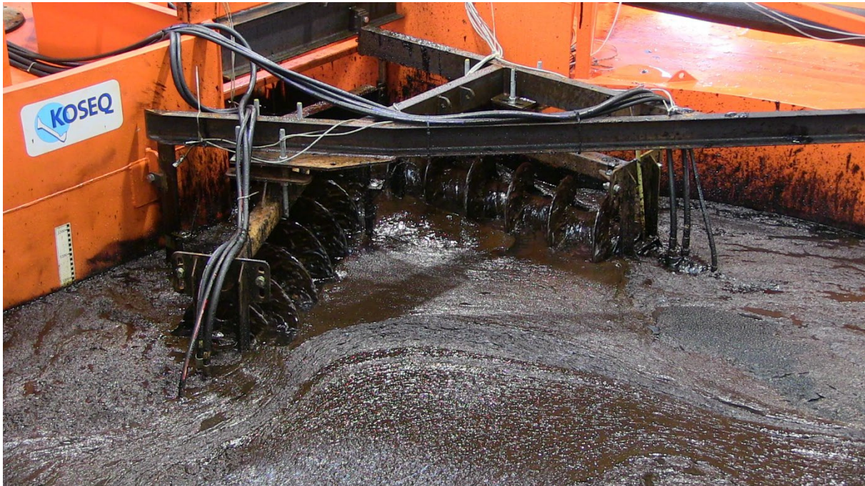
Figure 6: Photo of the Koseq modified Sweeping Arm weir skimmer operating in IM-29.
