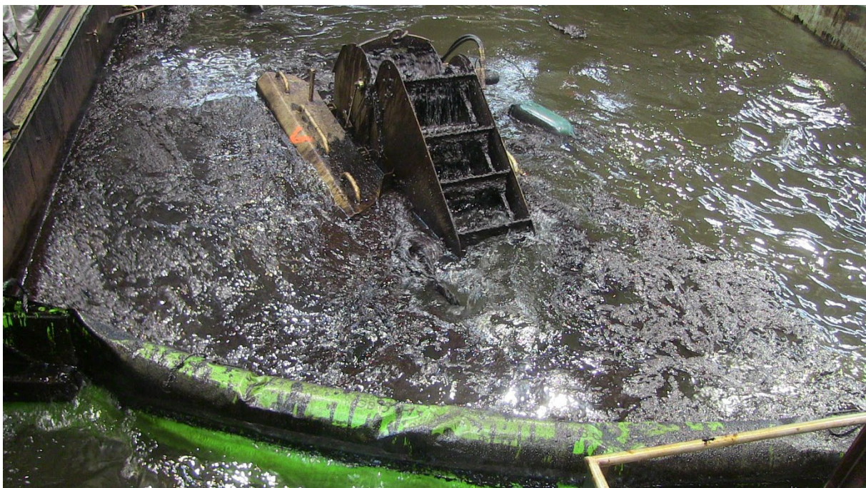
Figure 5: Photo of the Lamor LAM 50 skimmer with the feeder unit operating in the IM-28 oil.
