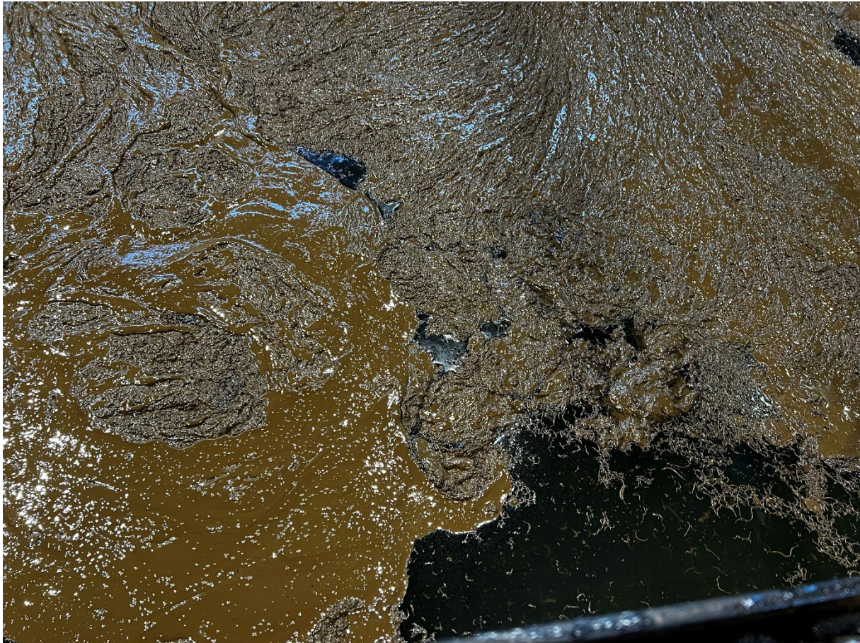
Figure 4: Photo of fragmentation/short properties of the IM-29 oil slick.
