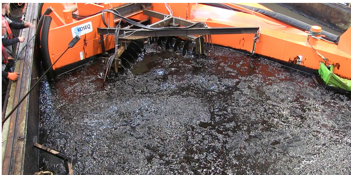
Figure 5: Photo of the Koseq modified Sweeping Arm weir skimmer operating in IM-28.
