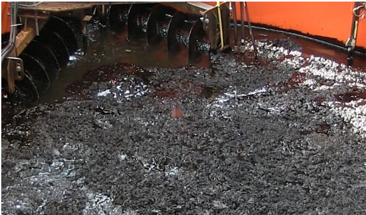
Figure 3: Photo showing that the IM-28 oil is bridging in front of skimmer.
