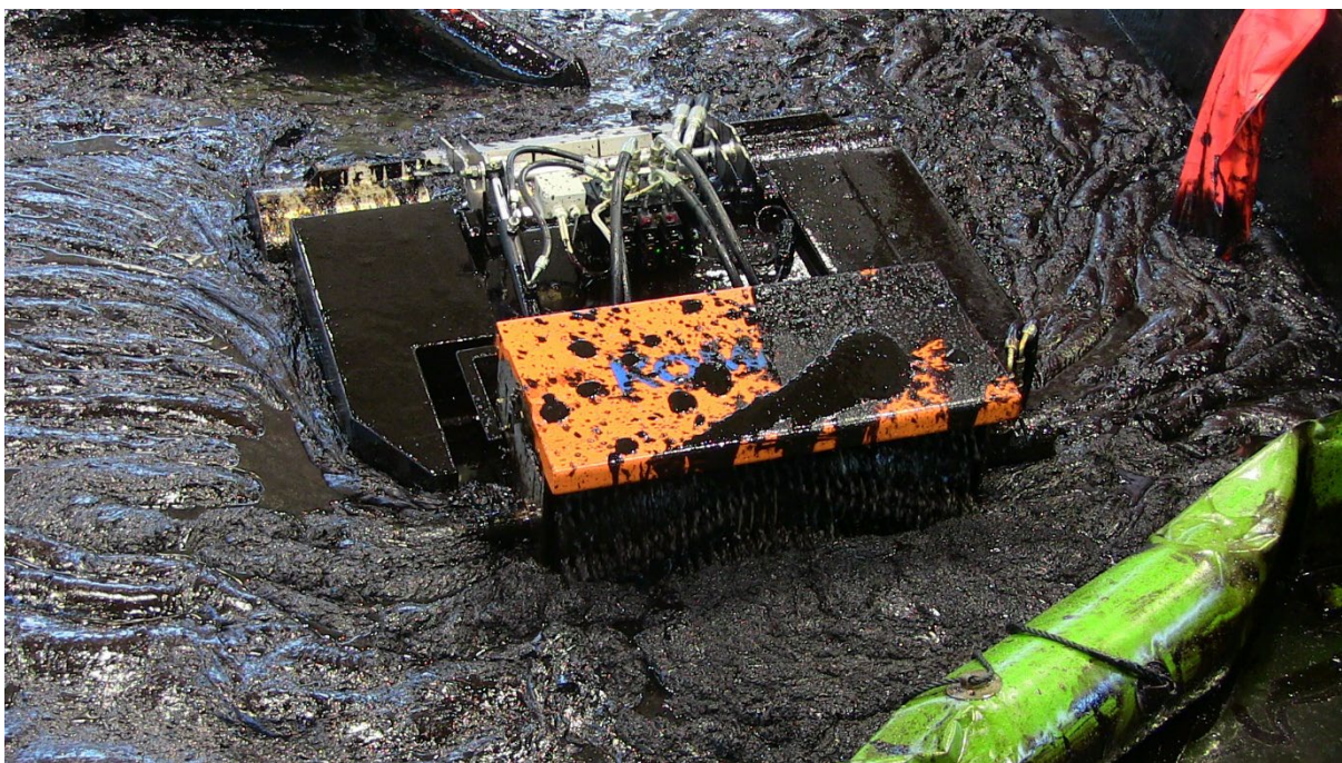
Figure 5: Photo of the Vikoma Komara Omni skimmer operating in the IM-28 oil.
