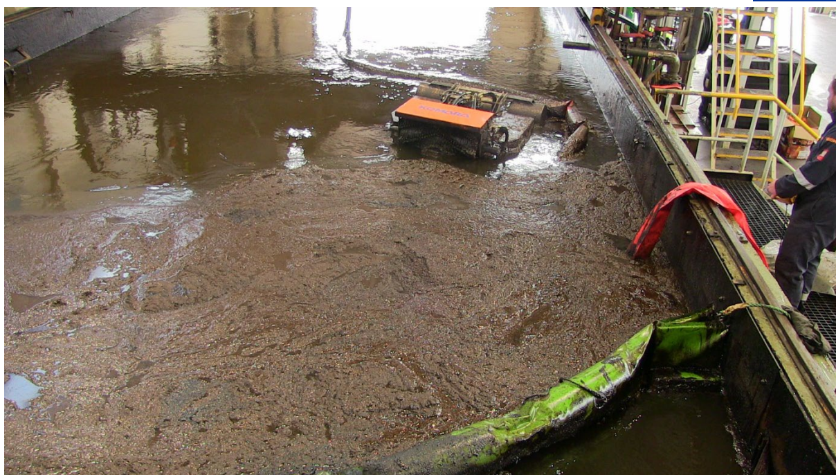
Figure 6: Photo of the Vikoma Komara Omni skimmer operating in the IM-29 oil.
