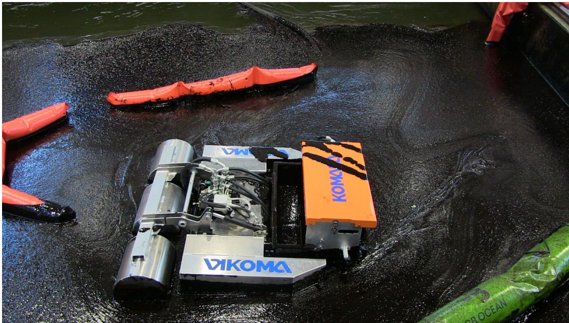
Figure 4: Photo of the Vikoma Komara Omni skimmer operating in the IM-27 oil.
