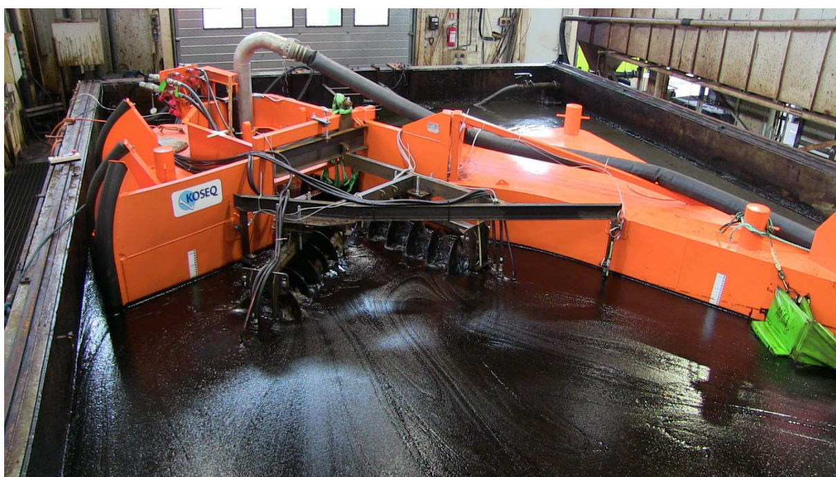
Figure 4: Photo of the Koseq modified Sweeping Arm weir skimmer operating in IM-27.
