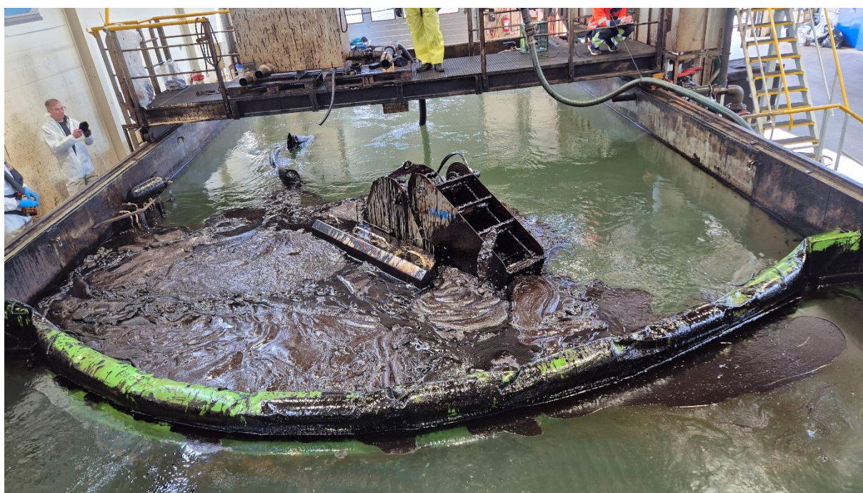
Figure 6: Photo of the Lamor LAM 50 skimmer with the feeder unit operating in the IM-29 oil.
