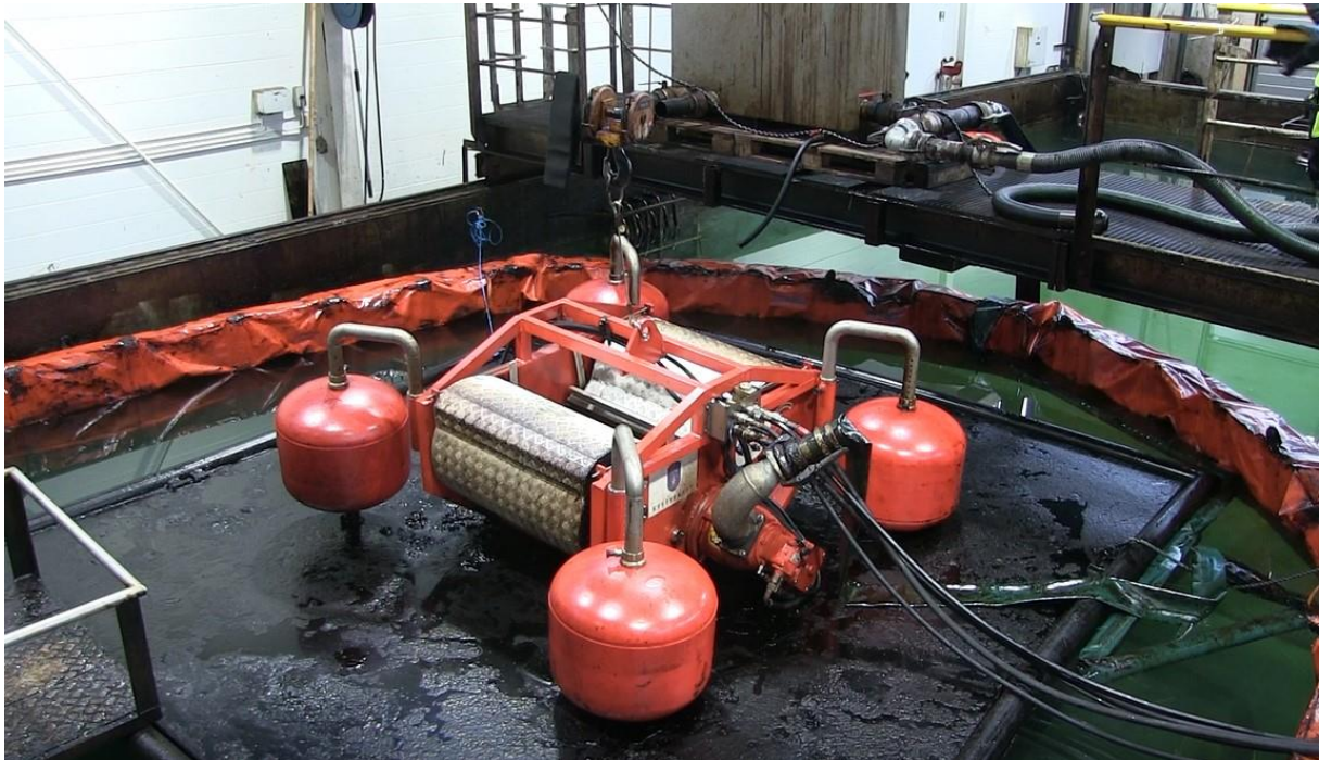
Figure 14: The drum skimmer stays on top of the oil. This skimmer weighs about 400 kg but did not manage to penetrate the oil slick.
