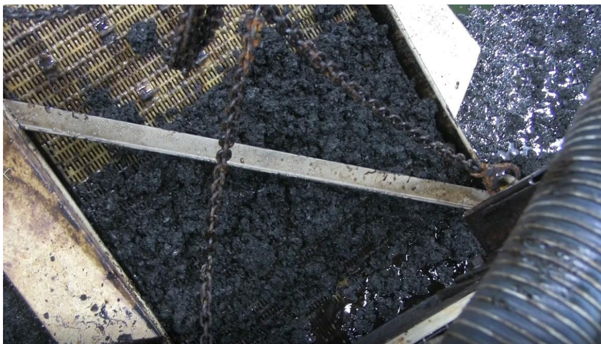
Figure 15: Belt skimmer collecting oil clumps of ULSFO IM-16. To get the skimmer to get hold of the clumps, it had to be actively moved towards the oil.
