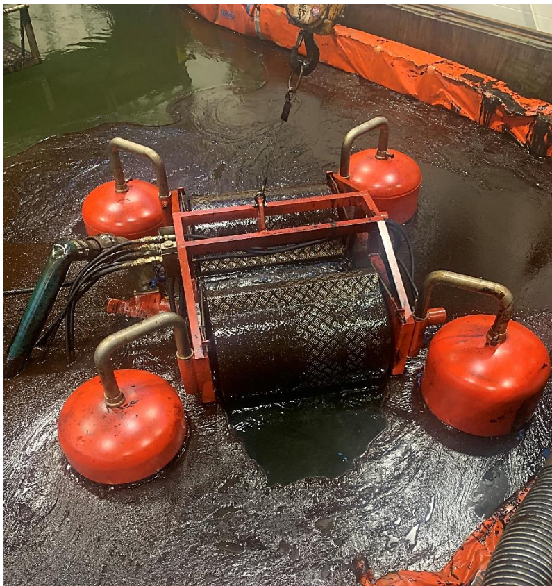
Figure 6: Photograph of the drum skimmer in motion in an attempt to take in oil. As the picture shows, there is still a clear area of water between skimmer and oil.
