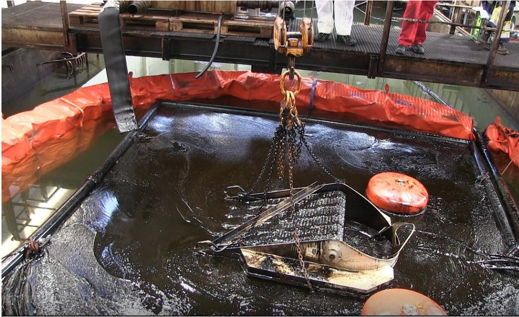
Figure 11: Photograph of the belt skimmer in fresh oil, showing the poor adhesion. The top of the belt has significantly less oil than the bottom, showing that the oil ran through the holes in the belt.
