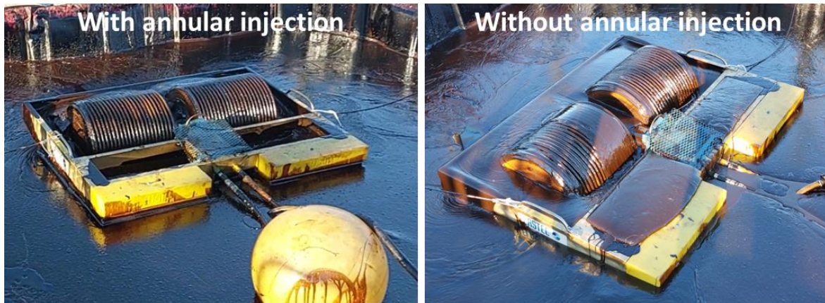
Figure 10 Emulsified IM-14 oil recovered with the drum skimmer, with and without water annular injection
