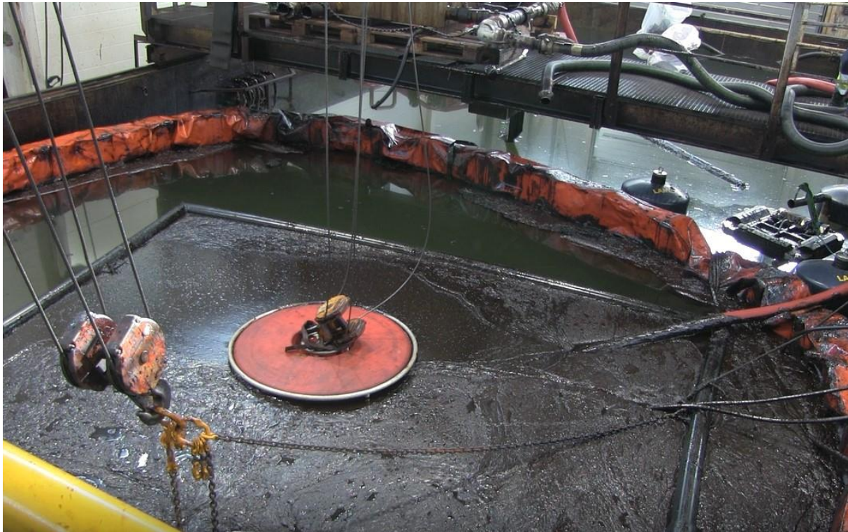
Figure 9: Photograph of weir skimmer in oil emulsion. There was no movement towards the skimmer, only water.
