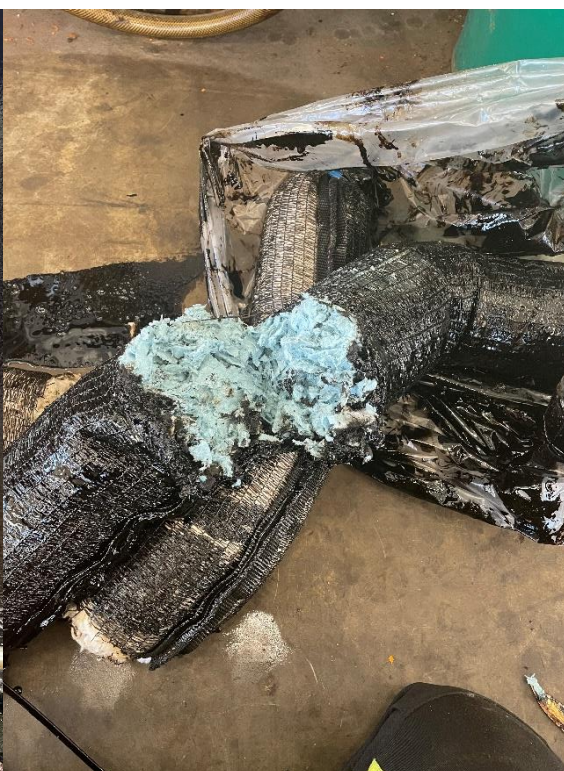
Figure 17: Cut polypropylene boom showing that neither oil nor water had penetrated the boom. This was also true for the cotton boom.
