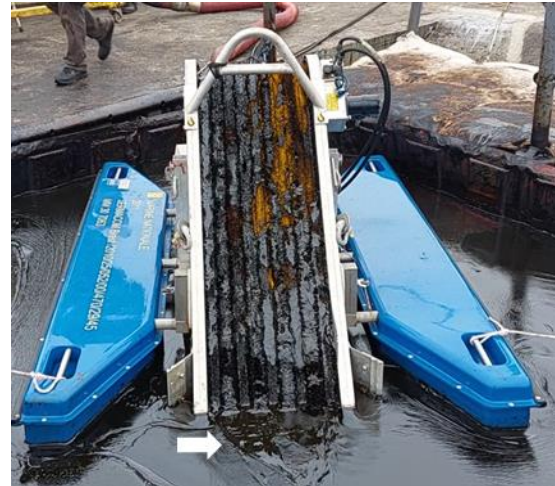
Figure 9 "Hole" in the fresh IM-14 oil slick created by the belt skimmer
