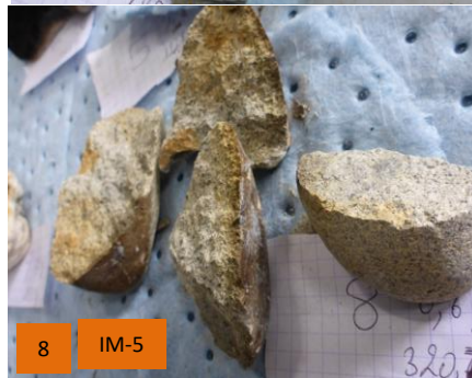
Pebbles broken after 7 days of contact with the oils
