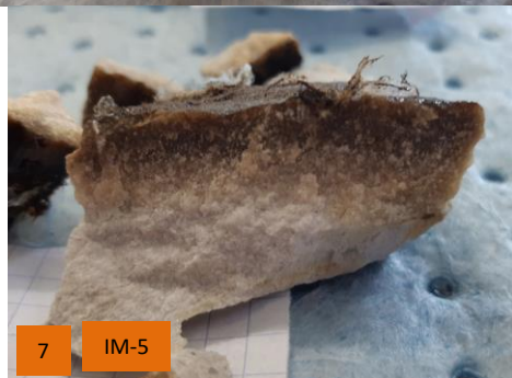
Pebbles broken after 3 days of contact with the oils
