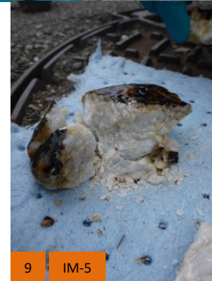
Pebbles broken after 14 days of contact with the oils
