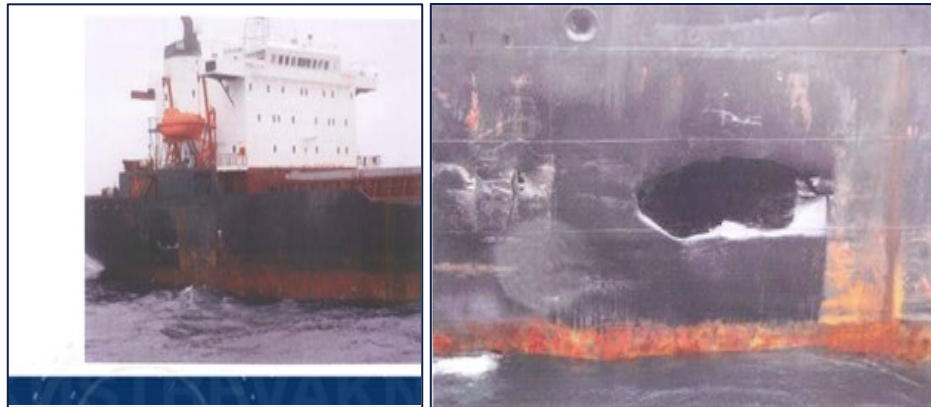
Golden Trader after the collision with the fishing vessel Vidar (Source: Kustbevakningen, 2011).
