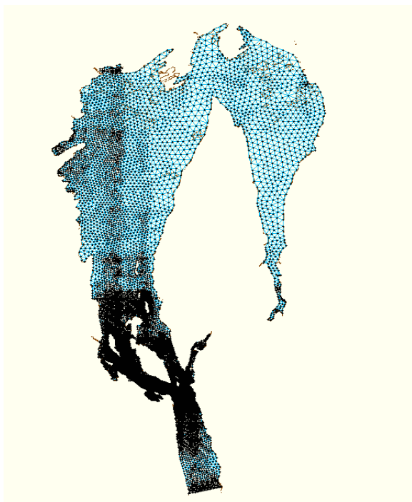
Figur 2-10: Mesh for Delft3d-analyser.
